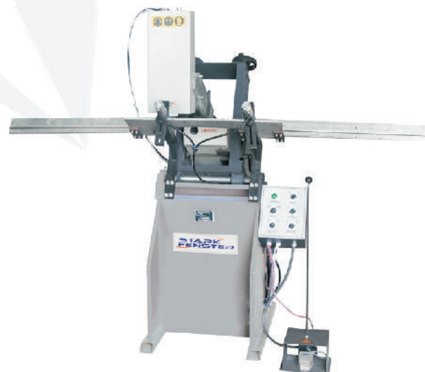
SCX02-2X60 uPVC PROFILE AUTO WATER-SLOT MILLING MACHINE
